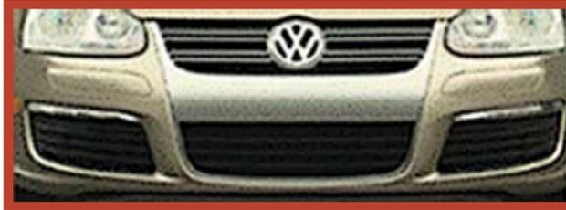
The chromium plating performed by Nicro Bolta (see sidebar) typically is used on the front grill of Volkswagen Jetta-Bora A-5.
