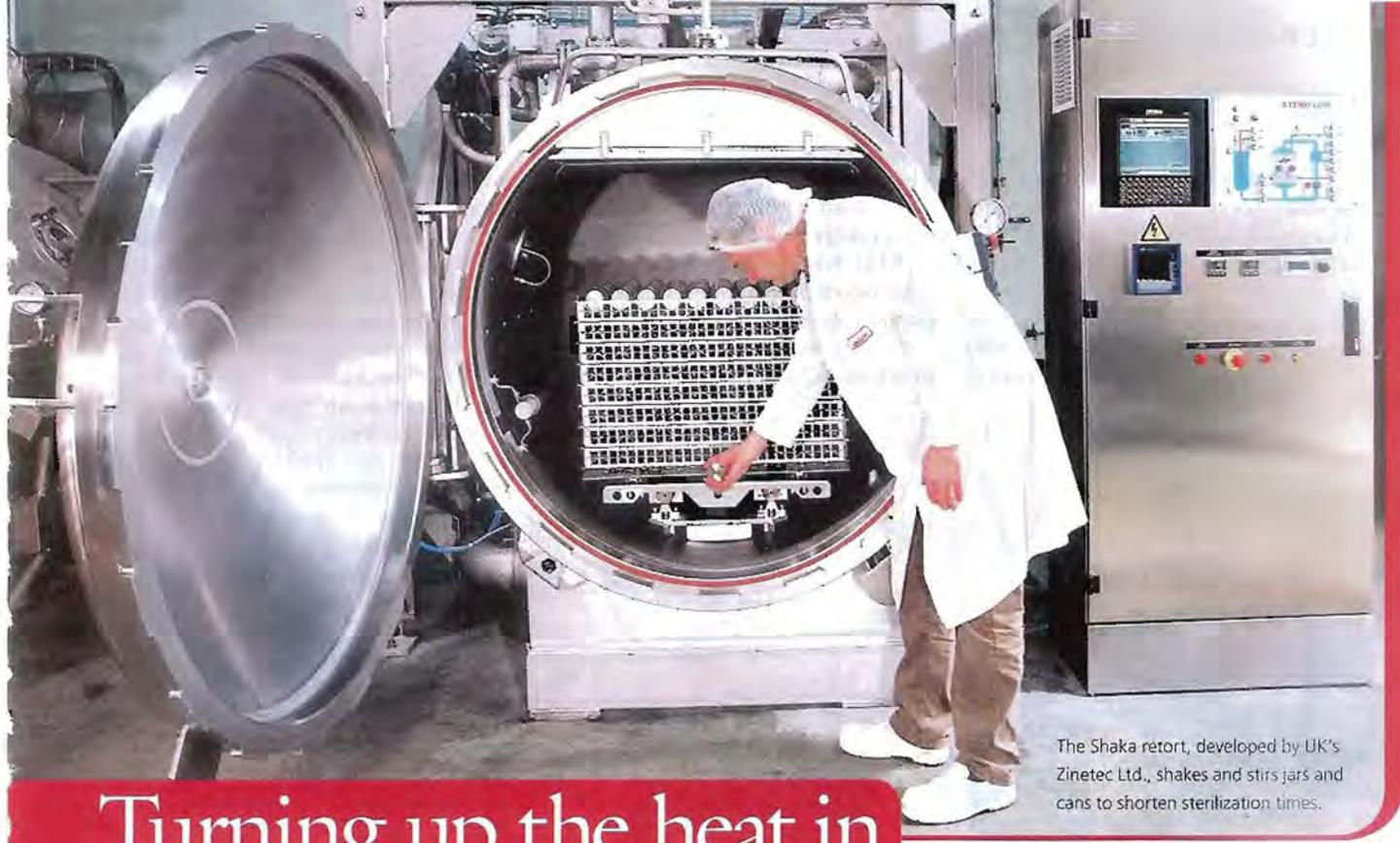
The Shaka retort, developed by UK's Zinetec Ltd., shakes and stirs jars and cans to shorten sterilization times.
