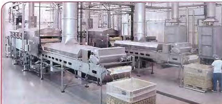
Heat and Control's HeatWave system conveys product through curtains of hot oil, claiming energy, cost and quality advantages over conventional "submerge-in-oil" frying.
