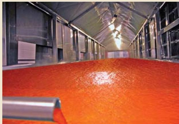
Cranberry slurry enters the MCD Technologies Model 2 RW dryer. The dryer is approximately 50-ft. long and six-ft. wide. Source: MCD Technologies.
